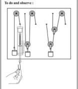
Step 1 :Place the hook of the Spring balance in the red coloured ring of the first system and pull it. Note the reading of the spring balance in newton.
